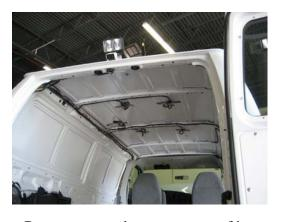
Be sure to tape harnesses to roof in approximate locations that accessories are being installed in Kwik kit. This will vary between the different model kits.
